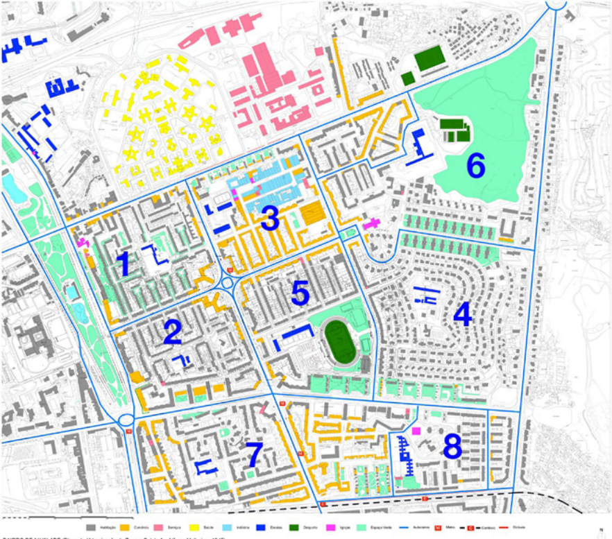
Fig. 4. António Carvalho, 2013, after Faria da Costa, General Plan of Alvalade Neighbourhood, 1945 . Each of the 8 urban cells of the Alvalade Plan is structured around a school (in blue) in the center. In orange colour are the main commercial/retail areas.
